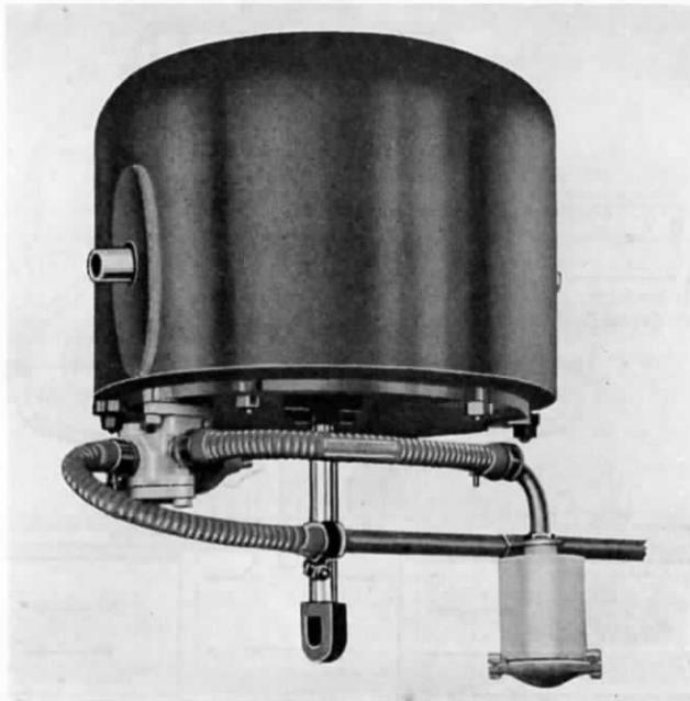
FIG. 189.—EXTERNAL VIEW OF WESTINGHOUSE QUICK-SERVICE VALVE.
