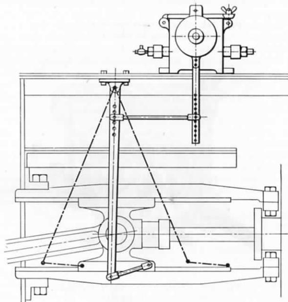
FIG. 217.—MECHANICAL LUBRICATOR DRIVEN FROM CROSSHEAD.
