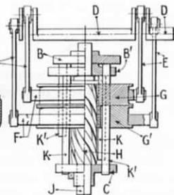
FIG. 110.—CAMSHAFT ASSEMBLY IN PLAN.
