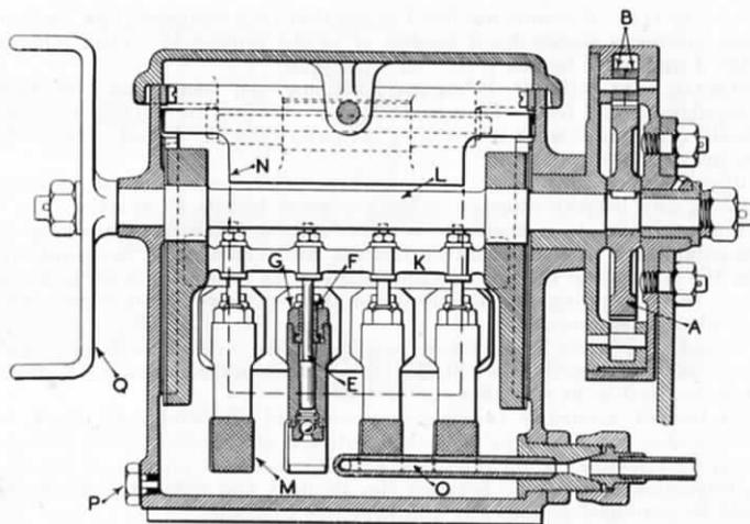
FIG. 229.—SILVERTOWN MECHANICAL LUBRICATOR IN SECTIONAL ELEVATION.
