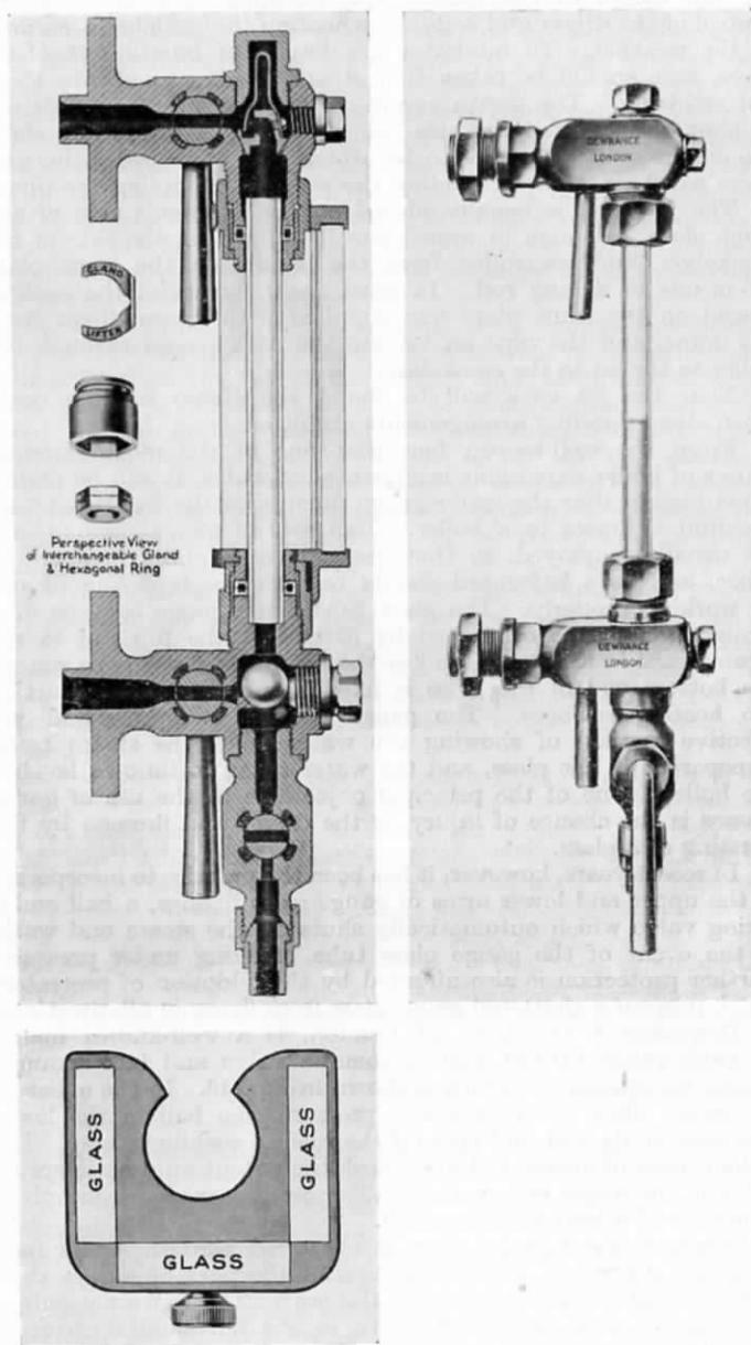
FIG. 46.—DETAILS OF DEWRANCE WATER-GAUGE FITTINGS FOR LOCOMOTIVES.
