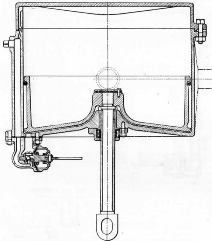
FIG. 184.—"C" TYPE CYLINDER (SEPARATE PATTERN).
