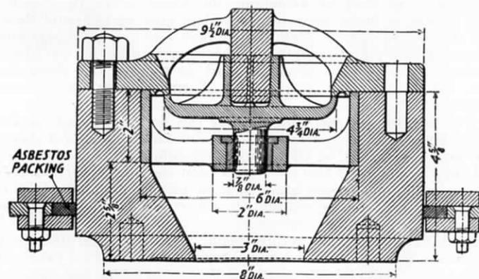
FIG. 163.—ANTI-VACUUM VALVE, L.N.E.R.
