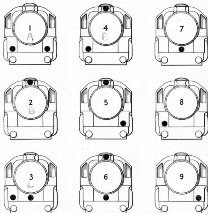
FIG. 11.—HEAD-LAMP CODE FOR CLASSIFYING TRAINS.
