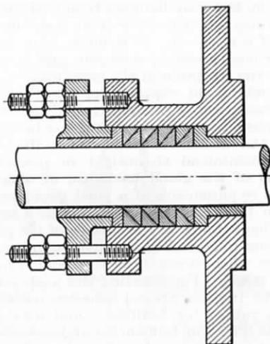
FIG. 117.—METALLIC PACKING FOR PISTON RODS.
