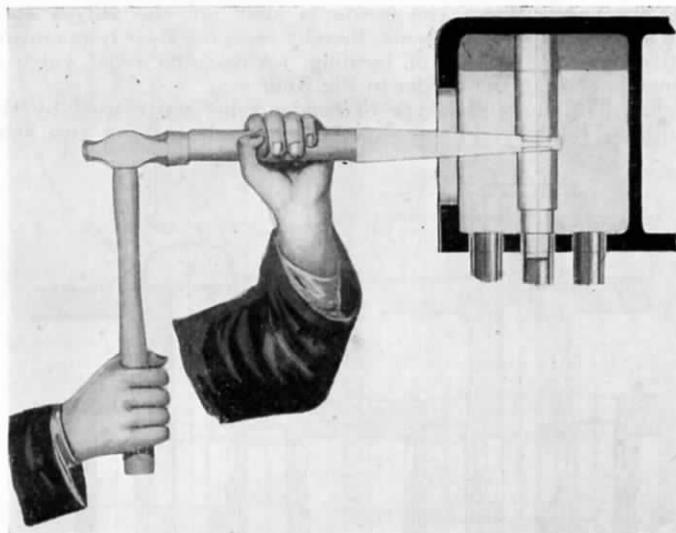
FIG. 168.—METHOD OF EXTRACTING SUPERHEATER TUBES.
