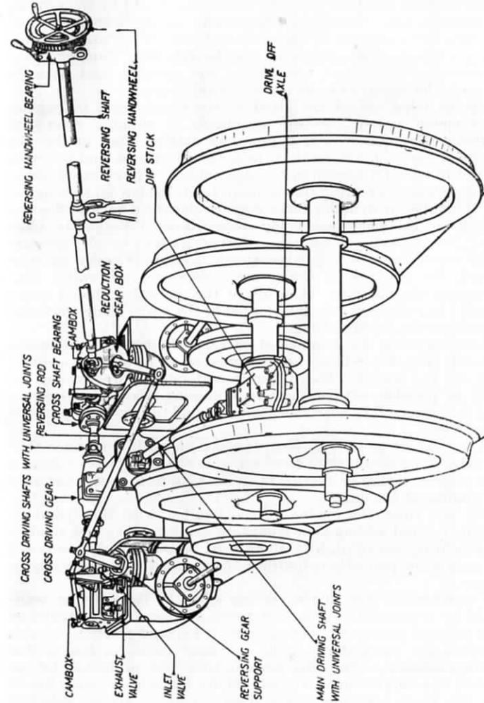
FIG. 112.—PERSPECTIVE VIEW OF CAPROTTI VALVE GEAR APPLIED TO A TWO-CYLINDER LOCOMOTIVE.
