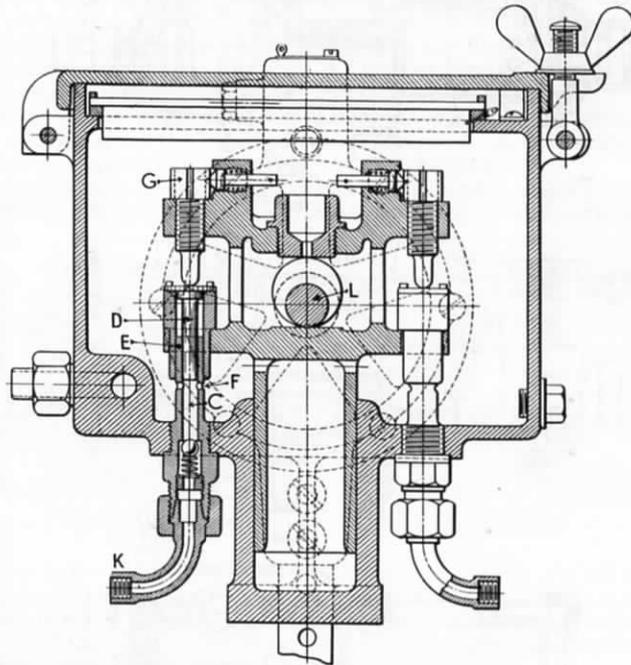
FIG. 225.—WAKEFIELD MECHANICAL LUBRICATOR (SINGLE-ACTING PATTERN).
