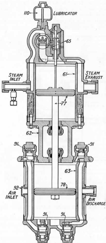
FIG. 200.—COMPRESSED AIR PUMP OF WESTINGHOUSE SYSTEM.
