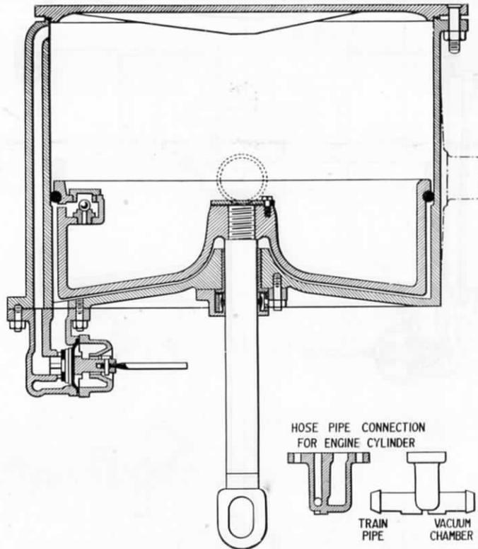
FIG. 185.—"E" TYPE CYLINDER (SEPARATE PATTERN).
