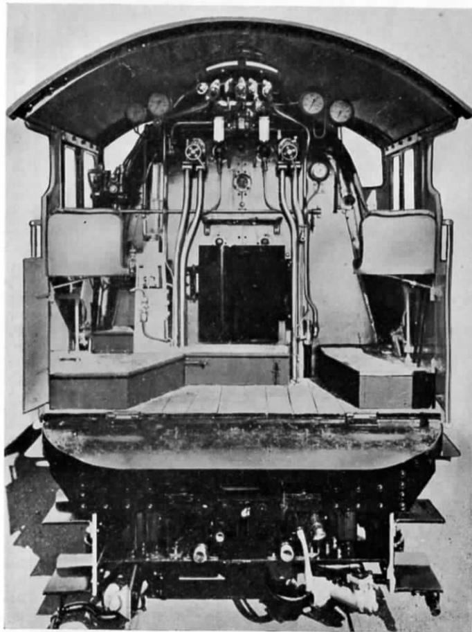
FIG. 62.—A MODERN LOCOMOTIVE CAB AND FITTINGS
