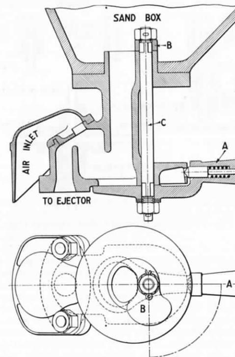
FIG. 79.—SECTION AND PLAN OF SANDBOX AND ATTACHMENTS.
