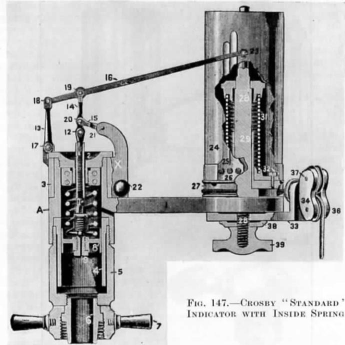
FIG. 147.—CROSBY "STANDARD" INDICATOR WITH INSIDE SPRING.
