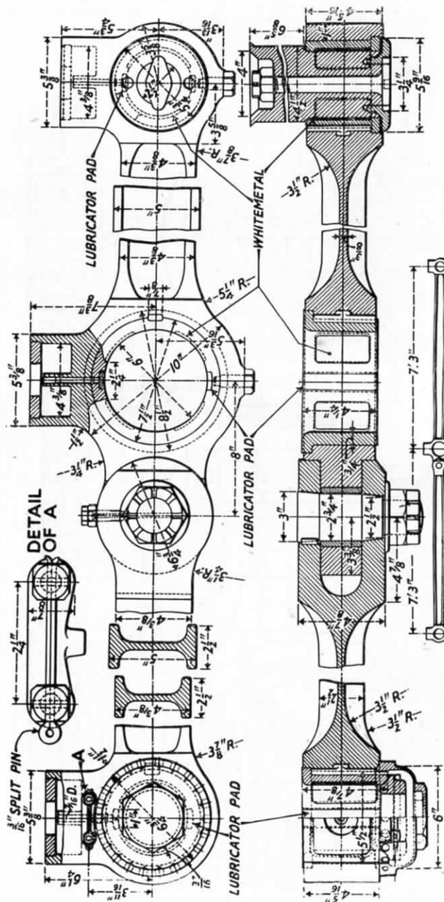
FIG. 88.—COUPLING ROD OF 4-6-2 TYPE (A4 CLASS) ENGINE, L.N.E.R.
