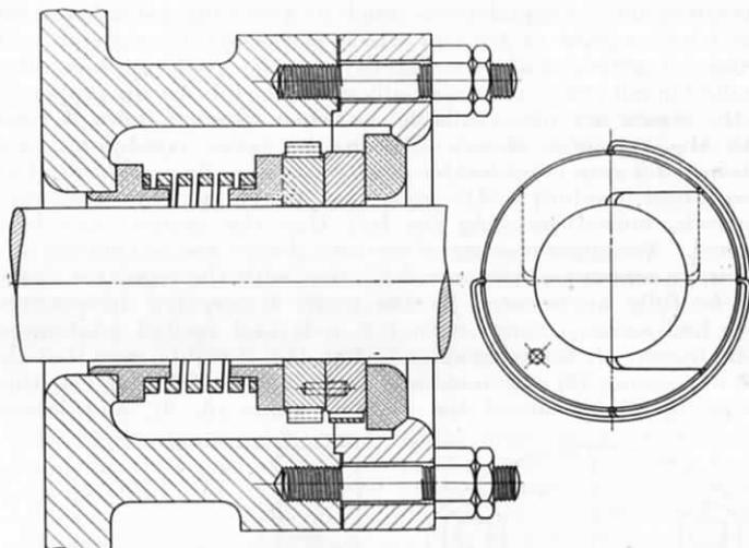
FIG. 122.—PACKING WITH CAST-IRON RINGS.
