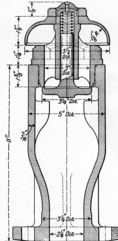
FIG. 173.—SUPERHEATER HEADER RELIEF VALVE, SOUTHERN RAILWAY.
