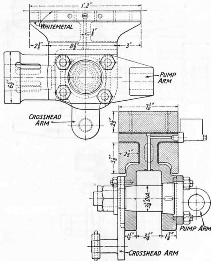
FIG. 124.—THREE SLIDE-BAR CROSSHEAD, SOUTHERN RAILWAY.
