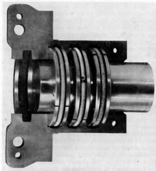
FIG. 120.—HOUSING FOR RINGS OF BRITIMP PACKING.
