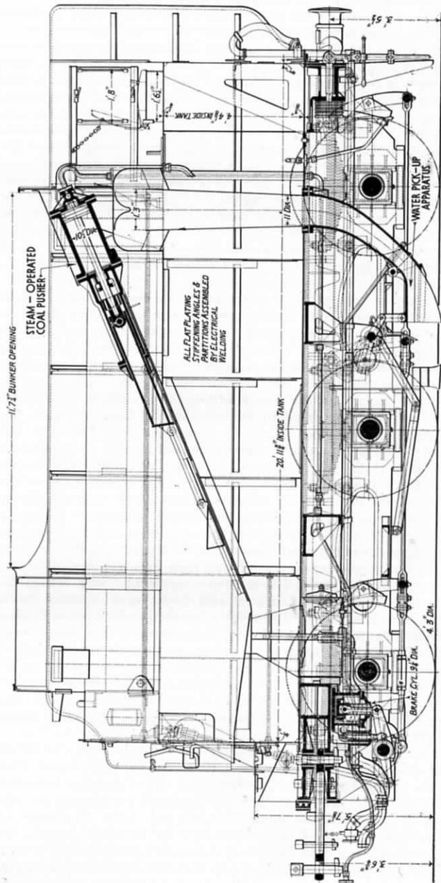
FIG. 178.—TENDER OF L.M.S.R. 4-6-2 TYPE STREAMLINED EXPRESS LOCOMOTIVE FITTED WITH WATER PICK-UP APPARATUS AND STEAM-OPERATED COAL PUSHER.
