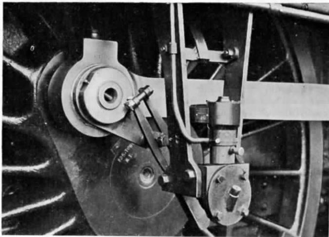
FIG. 251.—DRIVING GEAR AND GENERATOR.
