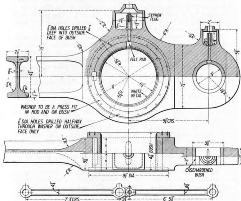
FIG. 84.—DETAILS OF COUPLING RODS OF 4-6-2 TYPE EXPRESS ENGINE, L.M.S.R.
