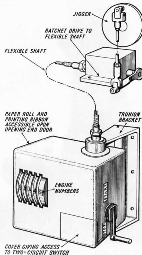
FIG. 15.—APPARATUS FOR RECORDING ENGINE NUMBER AND AMOUNT OF COAL DELIVERED TO TENDER.
