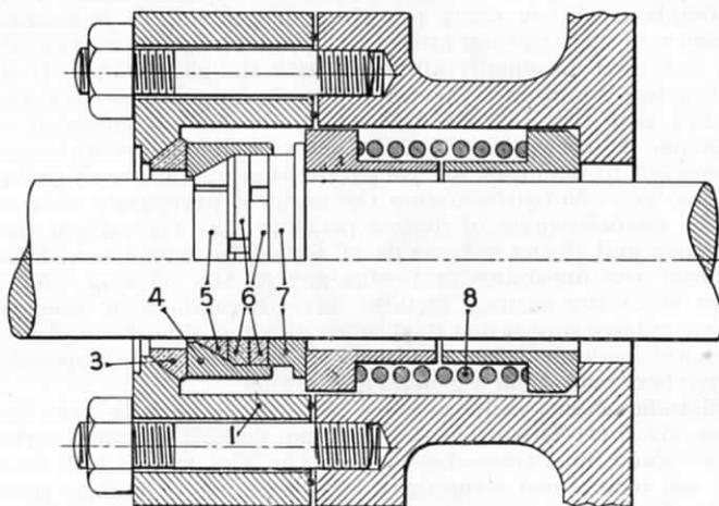
FIG. 118.—SPRING-CONTROLLED METALLIC PACKING.
