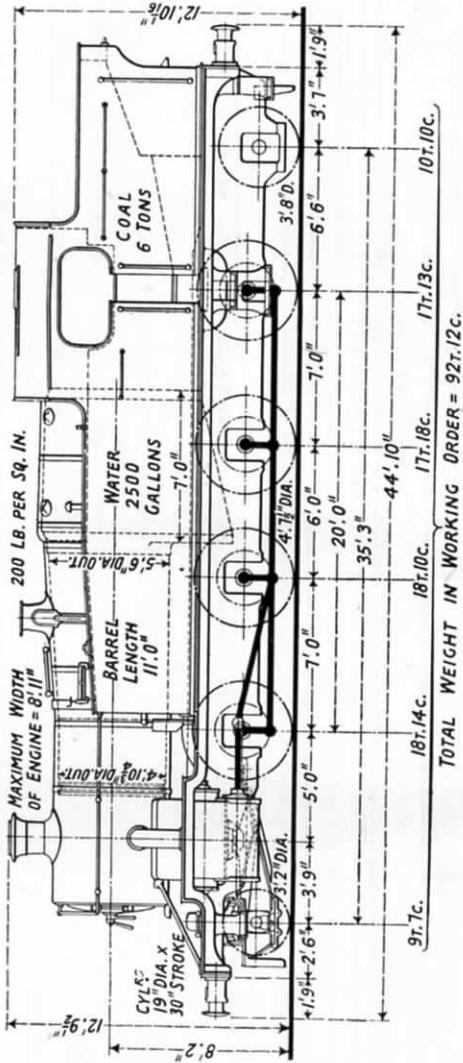
FIG. 288.—"7200" CLASS 2-8-2 TANK ENGINE, G.W.R.
