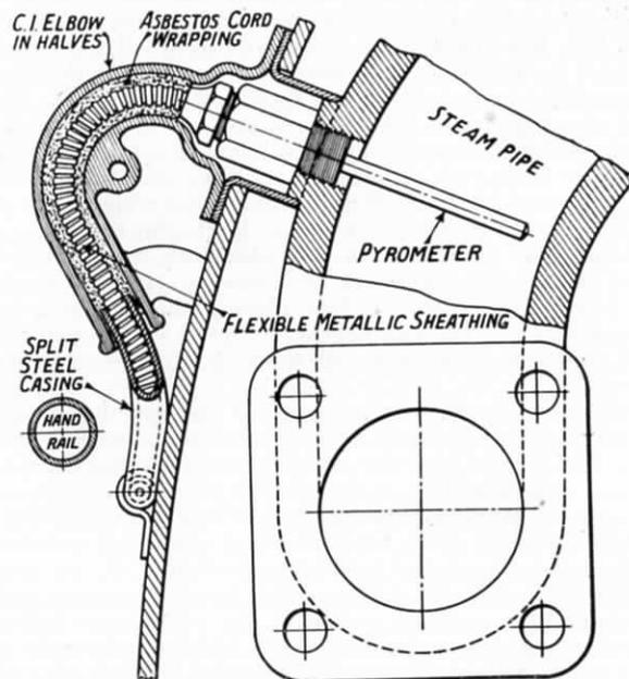
FIG. 176.—ARRANGEMENT OF THERMO-COUPLE
