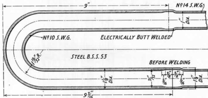
FIG. 172.—ELECTRICALLY BUTT-WELDED RETURN BEND OF "SWINDON" SUPERHEATER.
