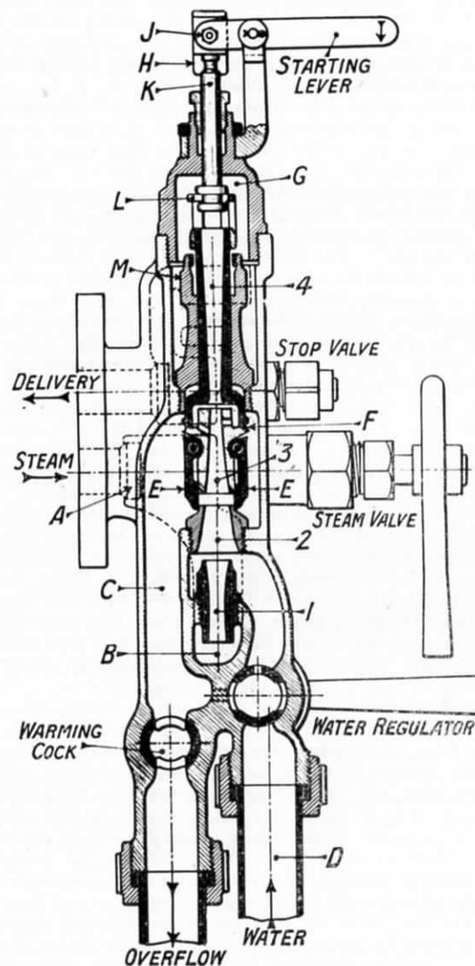
FIG. 52.—GRESHAM PATENT HOT-WATER COMBINATION INJECTOR.
