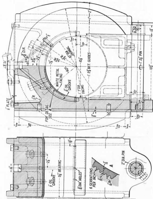
FIG. 66.—DRIVING AXLEBOX FOR MODERN ENGINES, L.M.S.R.
