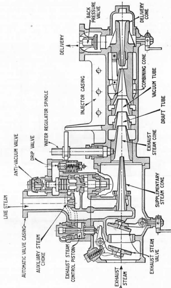
FIG. 54.—SECTION THROUGH EXHAUST-STEAM INLET AUTOMATIC VALVES AND INJECTOR NOZZLES.
