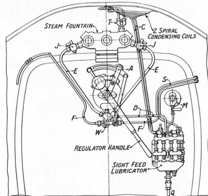
FIG. 232.—LUBRICATING FITTINGS IN CAB, G.W.R.
