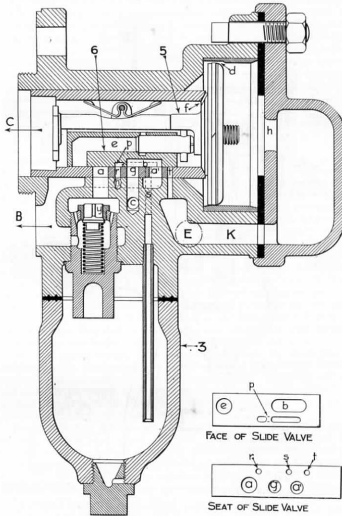
FIG. 206.—WESTINGHOUSE IMPROVED TRIPLE VALVE.
