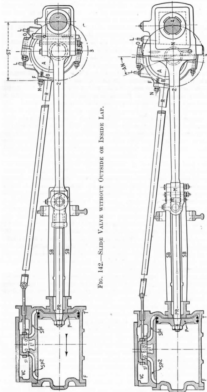
FIG. 142.—SLIDE VALVE WITHOUT OUTSIDE OR INSIDE LAP.
