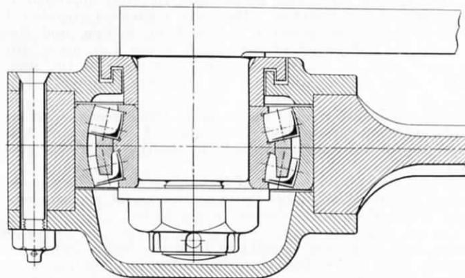
FIG. 77.—ROLLER-BEARING RETURN CRANK.
