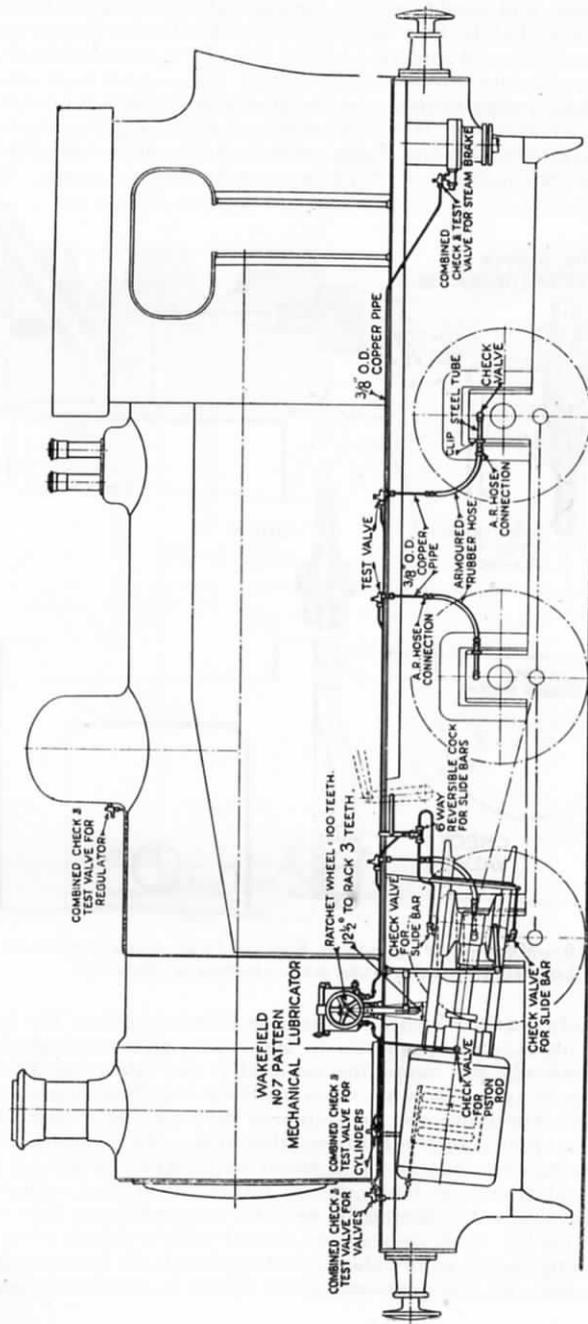
FIG. 220.—DIAGRAM OF LOCOMOTIVE EQUIPPED WITH THE WAKEFIELD MECHANICAL SYSTEM OF LUBRICATION.
