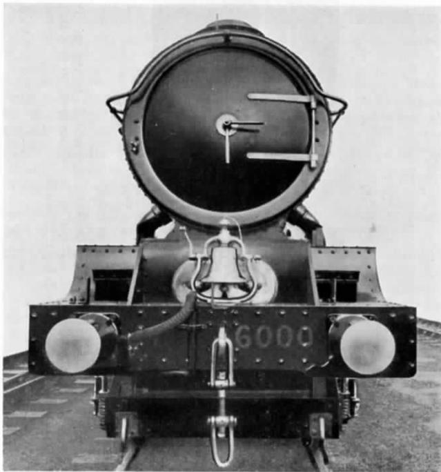
FIG. 268.—FRONT-END VIEW OF FOUR-CYLINDER 4-6-0 TYPE EXPRESS LOCOMOTIVE, No. 6000, King George V, G.W.R.
