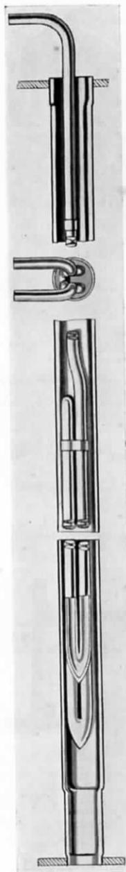
FIG. 164.—STANDARD "A" TYPE SUPERHEATER ELEMENT.
