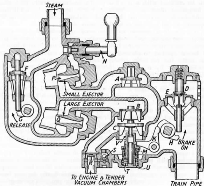
FIG. 192.—DIAGRAMMATIC VIEW OF "S.J." EJECTOR.
