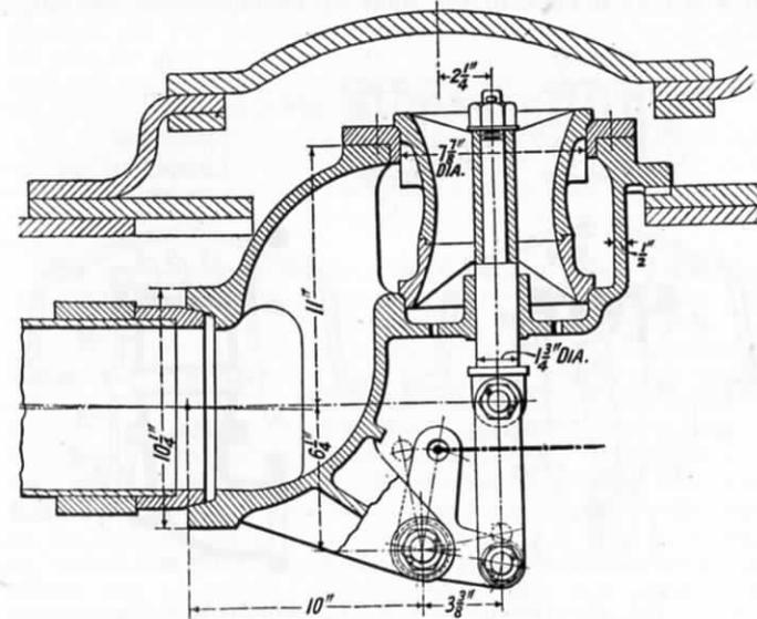
FIG. 40.—L.N.E.R. BALANCED REGULATOR VALVE.
