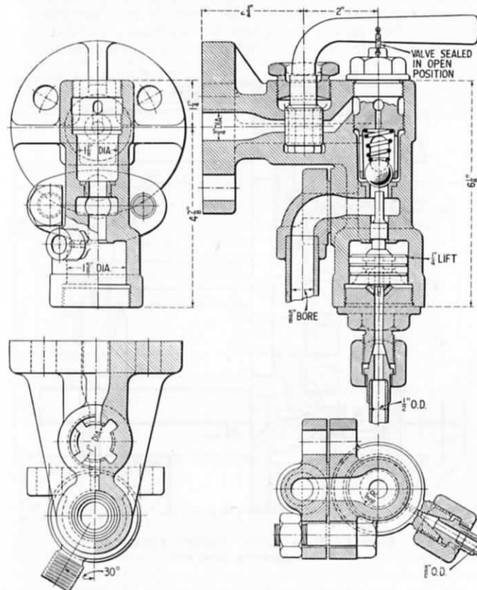
FIG. 43.—AUTOMATIC CONTINUOUS BLOWDOWN VALVE.
