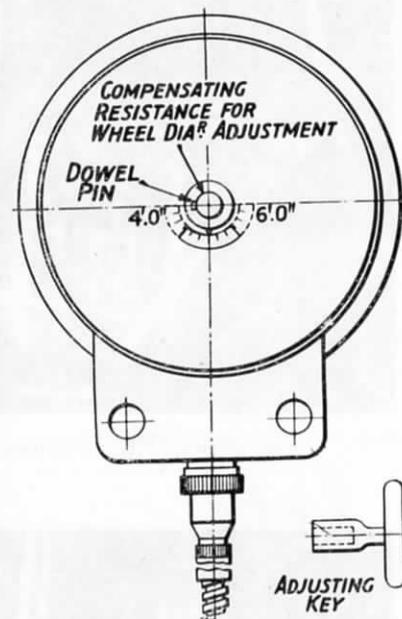
FIG. 249.—METHOD OF ADJUSTING TYRE WEAR, STONE-DEUTA ELECTRICAL SPEED INDICATOR.
