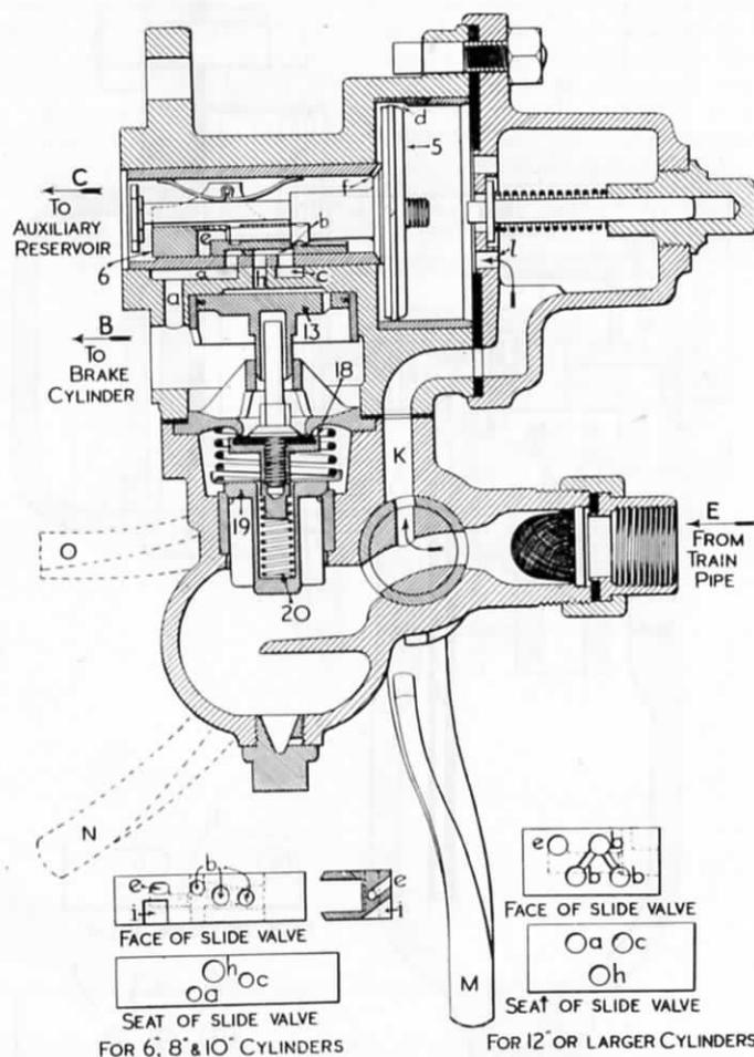
FIG. 205.—WESTINGHOUSE QUICK-ACTING TRIPLE VALVE.
