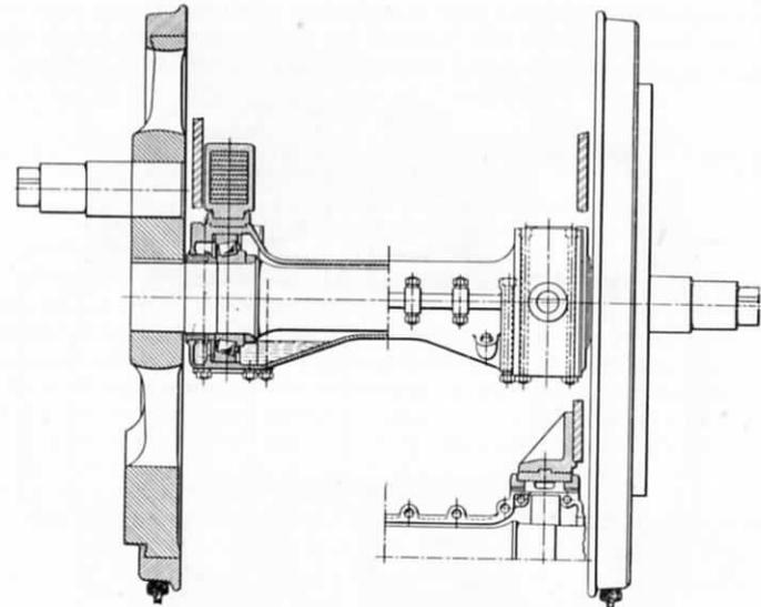
FIG. 71.—TIMKEN "CANNON" TYPE AXLEBOX FOR LOCOMOTIVE DRIVING AXLES. SINGLE TAPERED ROLLER BEARING MOUNTED ON EACH JOURNAL, HOUSED IN TUBULAR-TYPE AXLEBOX, EMBRACING THE ENTIRE AXLE BETWEEN WHEEL HUBS.
