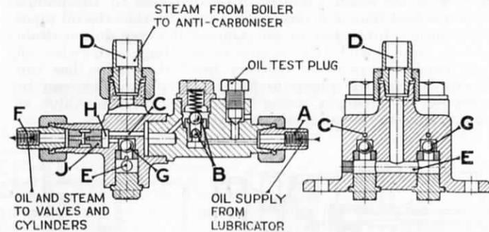
FIG. 226.—ANTI-CARBONISER (WAKEFIELD PATTERN).
