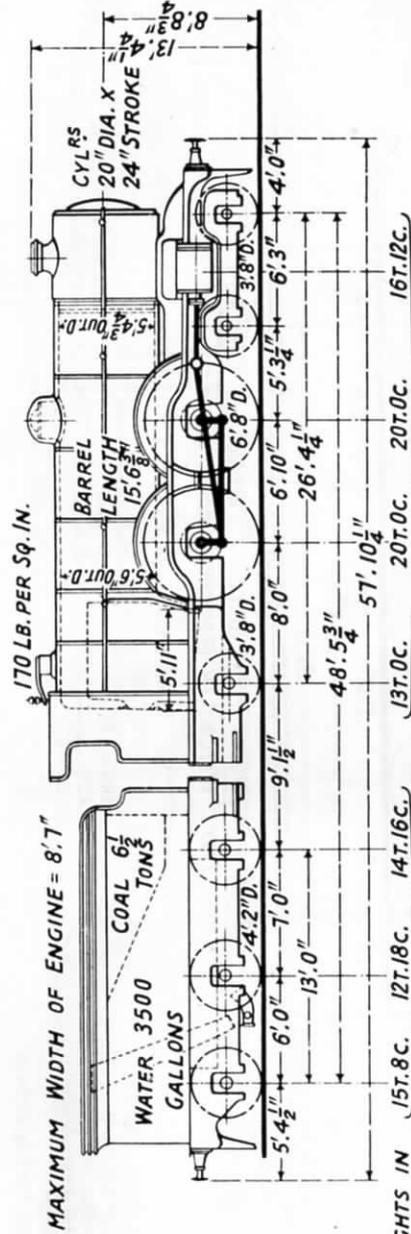
FIG. 291.—"C1" CLASS 4-4-2 LOCOMOTIVE, L.N.E.R.
