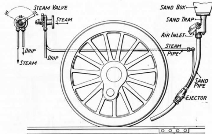
FIG. 78.—ARRANGEMENT OF STEAM SANDING GEAR FOR LOCOMOTIVES.
