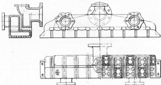
FIG. 161.—TYPE "A.X." SUPERHEATER HEADER.
