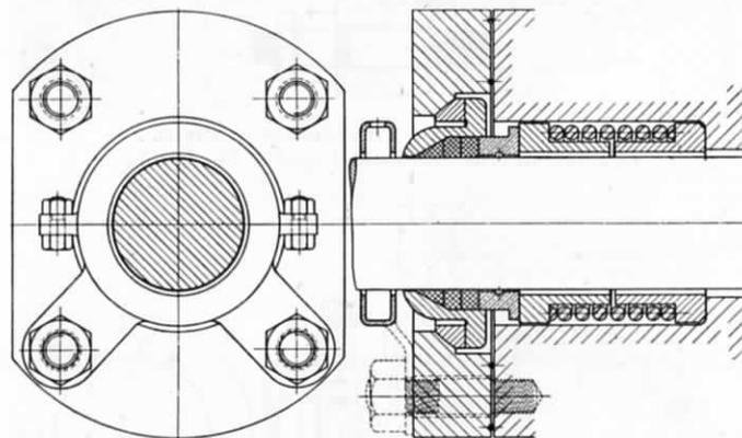
FIG. 121.—UNITED STATES METALLIC PACKING (AIR-COOLED TYPE).
