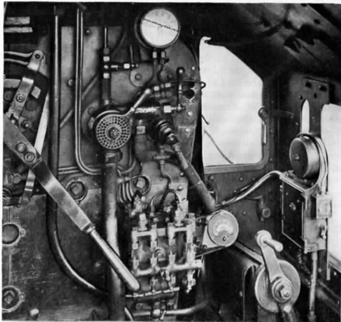
FIG. 250.—G.W.R. SPEEDOMETER, CAB FITTINGS.
