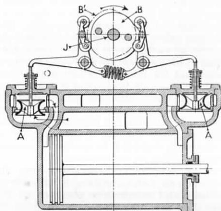
FIG. 107.—SECTION THROUGH CYLINDER AND INLET VALVES.
