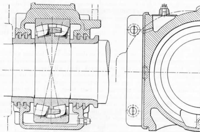
FIG. 73.—S.K.F. ROLLER-BEARING AXLEBOX FOR INSIDE JOURNALS.
