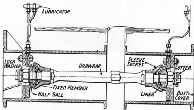
FIG. 271.—DETAILS OF GOODALL ARTICULATED DRAWGEAR FOR LOCOMOTIVES (BOLTED PATTERN).
