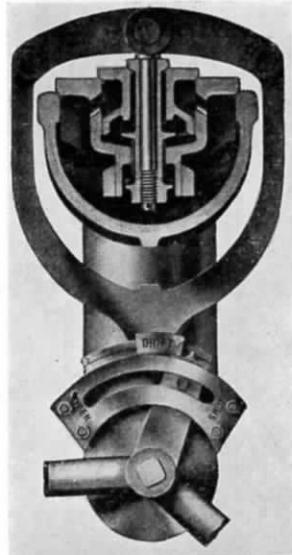
FIG. 38.—THE "JOCO" COMBINED REGULATOR AND DRIFTING VALVE.
