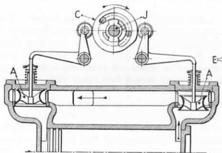
FIG. 108.—SECTION THROUGH EXHAUST VALVES.
