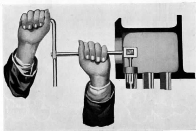
FIG. 167.—METHOD OF EXPANDING SUPERHEATER TUBES.
