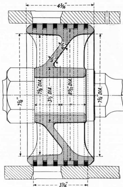
FIG. 102.—LATEST TYPE OF PISTON VALVE, L.M.S.R.
