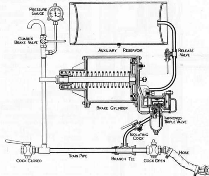
FIG. 199.—GENERAL ARRANGEMENT OF WESTINGHOUSE AIR BRAKE EQUIPMENT ON TRAIN.
