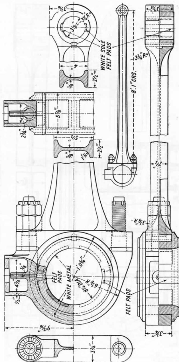
FIG. 135.—INSIDE CONNECTING ROD, L.N.E.R.
