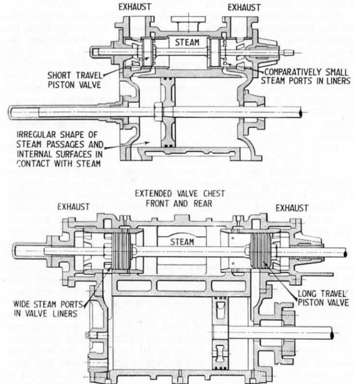
FIG. 99.—ABOVE: OLD PATTERN CYLINDER AND VALVE. BELOW: CYLINDER VALVE AND PISTON OF NEW STANDARD LOCOMOTIVES, L.M.S.R.
