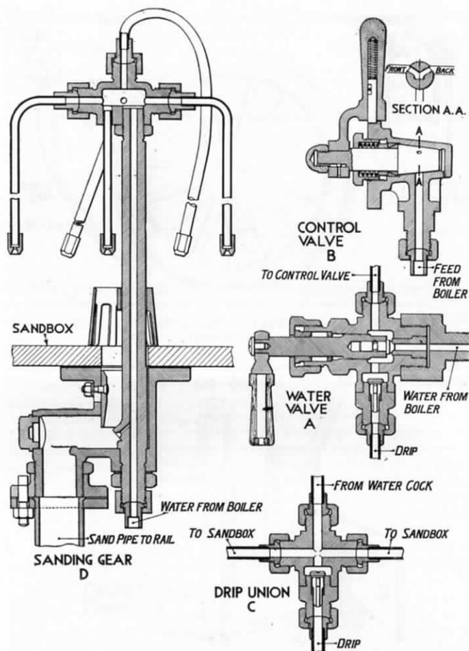
FIG. 80.—DETAILS OF LAMBERT WET SANDING GEAR.
