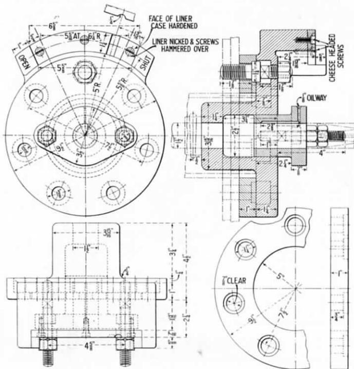
FIG. 233.—DETAILS OF STUFFING-BOX AND OTHER FITTINGS, G.W.R.
