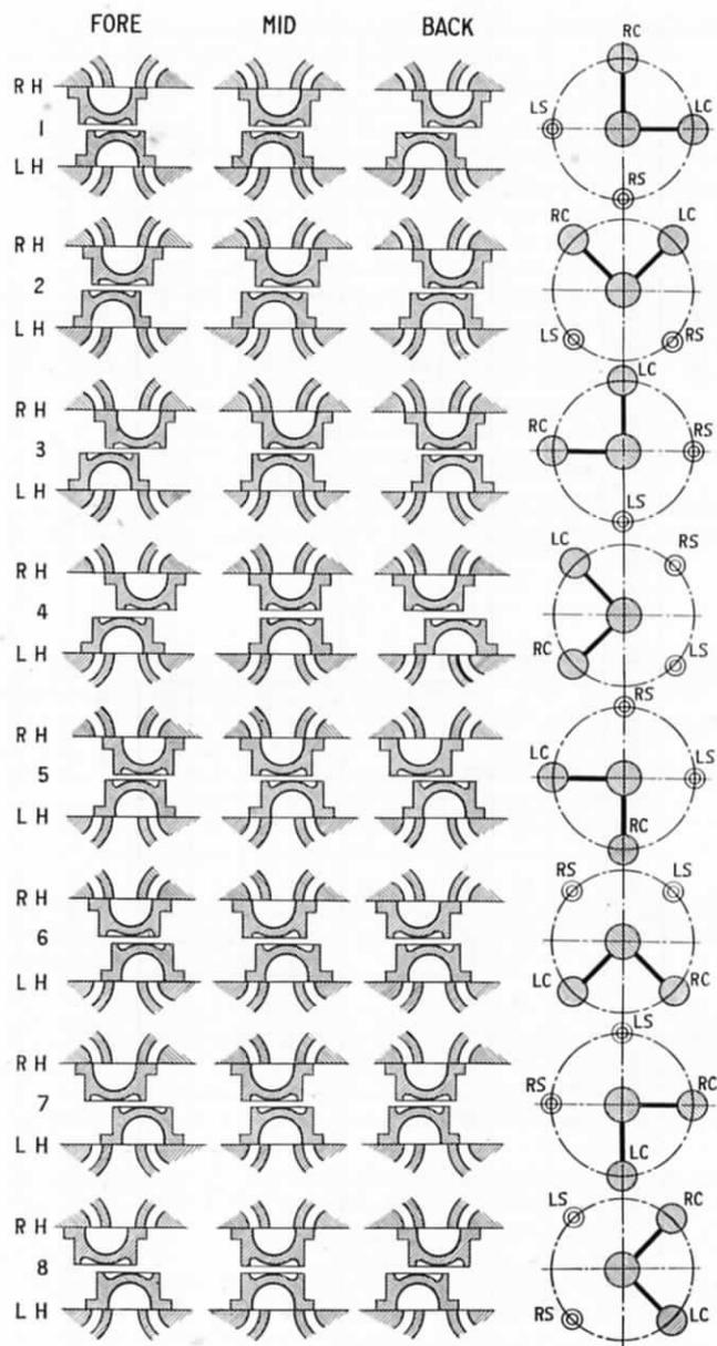
FIG. 258.—RELATIVE POSITIONS OF CRANKS, VALVES, AND SLIDE RODS.
