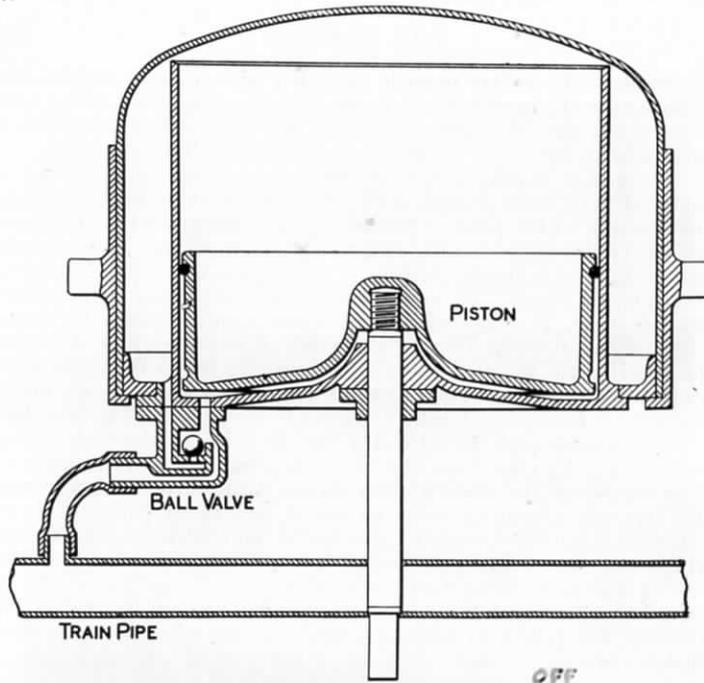
FIG. 181.—AUTOMATIC VACUUM BRAKE, "OFF."
