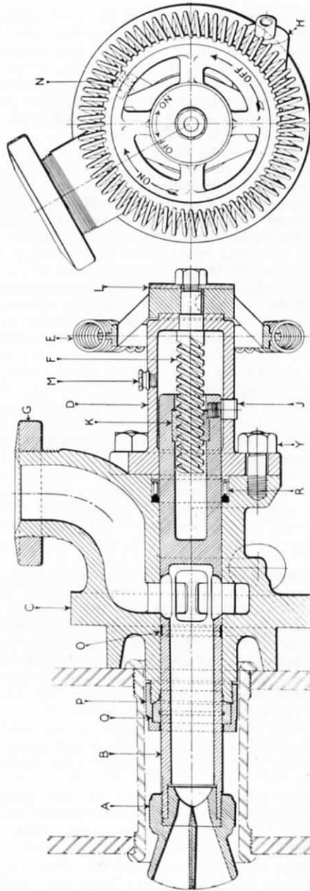
FIG. 21.—CLYDE PATENT SOOT BLOWER FOR FITTING TO BACK OF FIREBOX.
