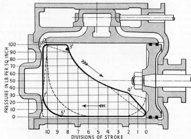
FIG. 150.—INDICATOR DIAGRAM SUPERIMPOSED ON LOCOMOTIVE CYLINDER SHOWING ACTION OF STEAM.
