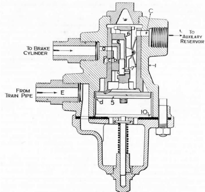
FIG. 204.—WESTINGHOUSE "ORDINARY" TRIPLE VALVE.
