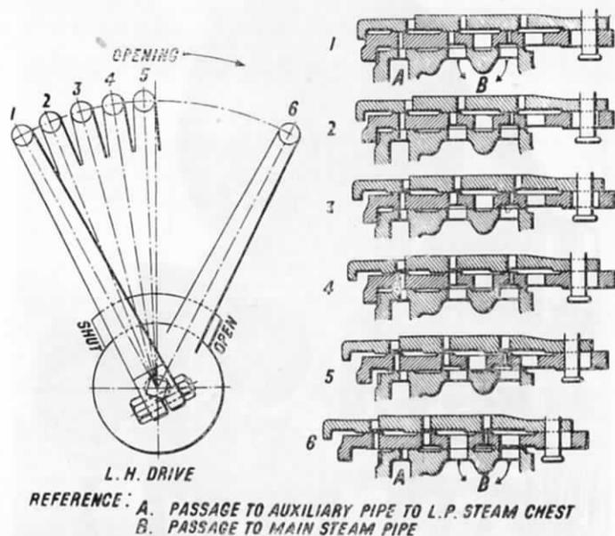
FIG. 157.—DIAGRAM SHOWING METHOD OF ADMITTING LIVE STEAM TO L.P. CYLINDERS, COMPOUND LOCOMOTIVE, L.M.S.R.
