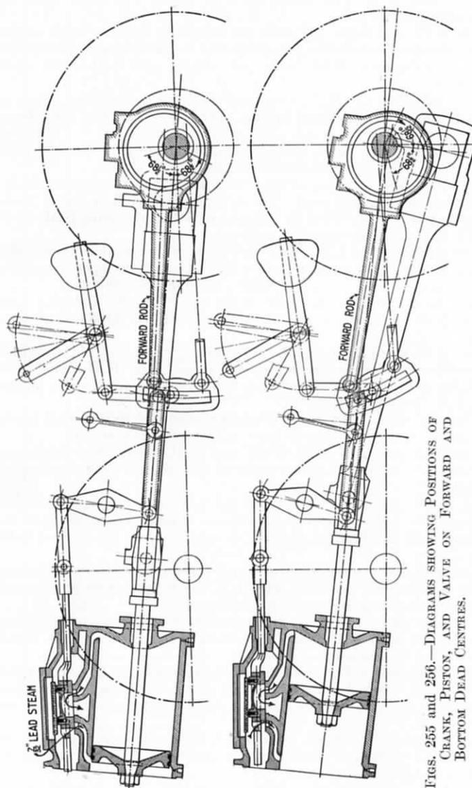
FIGS. 255 AND 256.—DIAGRAMS SHOWING POSITIONS OF CRANK, PISTON, AND VALVE ON FORWARD AND BOTTOM DEAD CENTRES.
