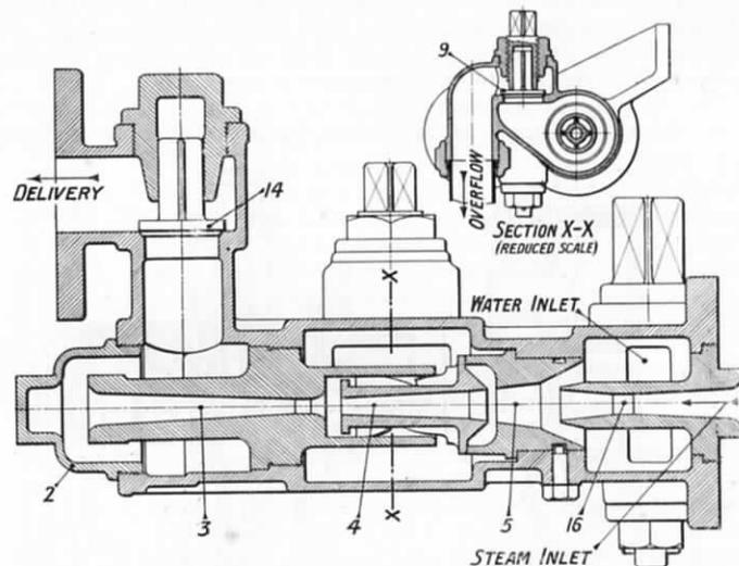
FIG. 51.—GRESHAM UNDER-FOOTPLATE TYPE INJECTOR.
