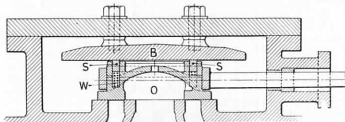
FIG. 101.—RICHARDSON BALANCED SLIDE VALVE
