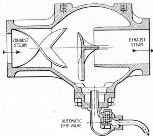
FIG. 59.—SECTION THROUGH GREASE SEPARATOR AND DRIP VALVE.
