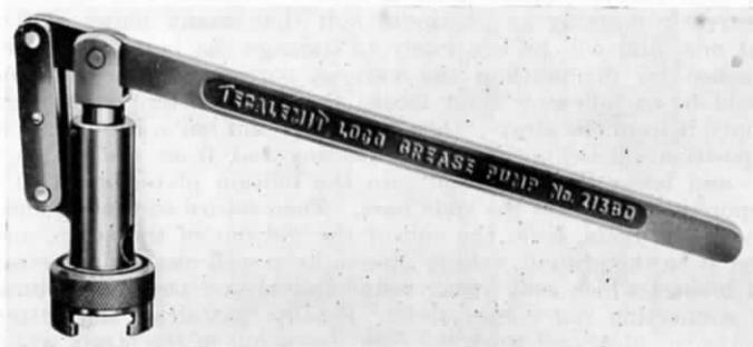
FIG. 136.—GUN FOR TECALEMIT HARD-GREASE LUBRICATION.
