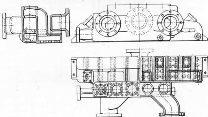
FIG. 162.—THE "MeLeSCO" MULTIPLE VALVE REGULATOR.
