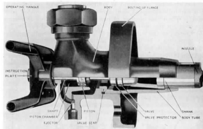
FIG. 18.—DIAMOND SOOT BLOWER: VALVE OPEN.
