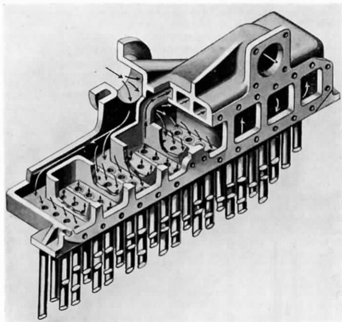
FIG. 166.—ELEMENTS EXPANDED DIRECT INTO HEADER.
