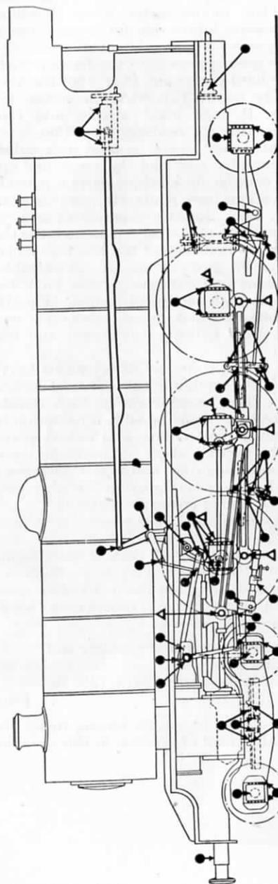
FIG. 139.—DIAGRAM OF LOCOMOTIVE SHOWING POINTS ADAPTABLE FOR GREASE LUBRICATION, TECALEMIT SYSTEM.
