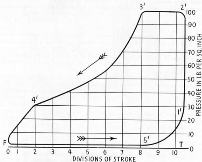
FIG. 149.—DIAGRAM TAKEN FROM ENGINE AT LOW SPEED.
