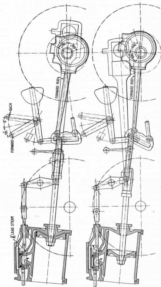
FIGS. 253 AND 254.—DIAGRAMS SHOWING RELATIVE CRANK, PISTON, AND VALVE POSITIONS IN FORWARD GEAR (BACK AND TOP DEAD CENTRES).
