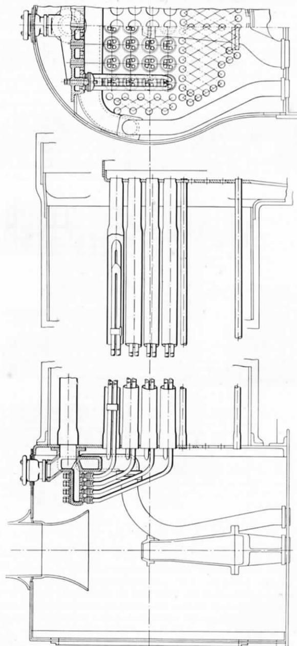
FIG. 160.—GENERAL ARRANGEMENT OF SMOKETUBE TYPE SUPERHEATER WITH BALL-JOINT ELEMENTS AND VACUUM RELIEF VALVE.
