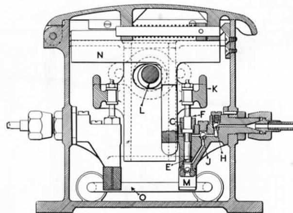
FIG. 230.—SILVERTOWN MECHANICAL LUBRICATOR IN CROSS-SECTION.
