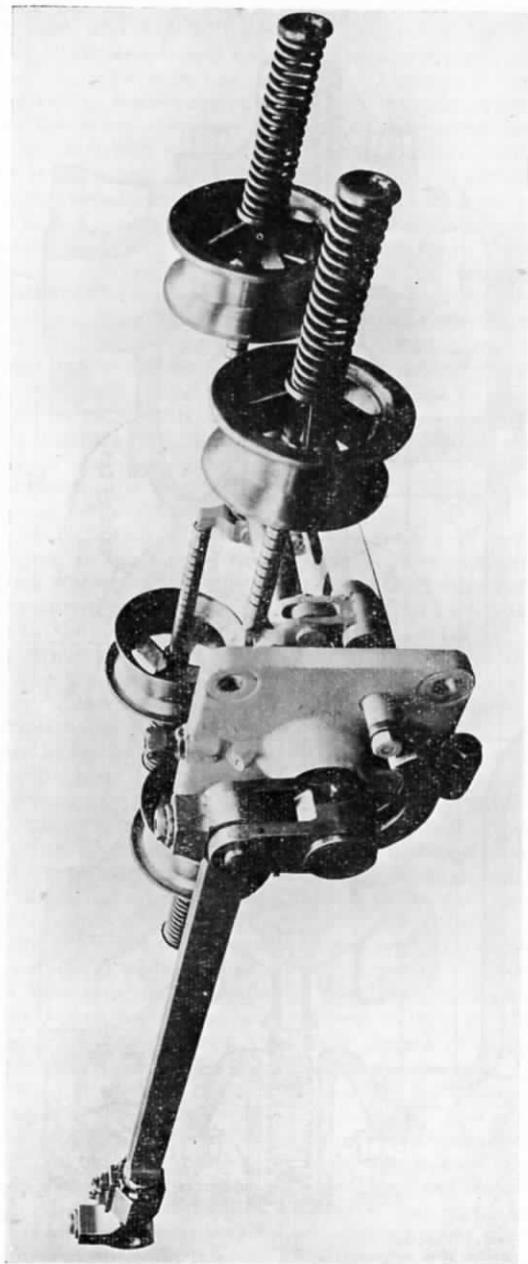
FIG. 104.—ARRANGEMENT OF POPPET VALVES AND LEVERS; "O.C." TYPE GEAR.
