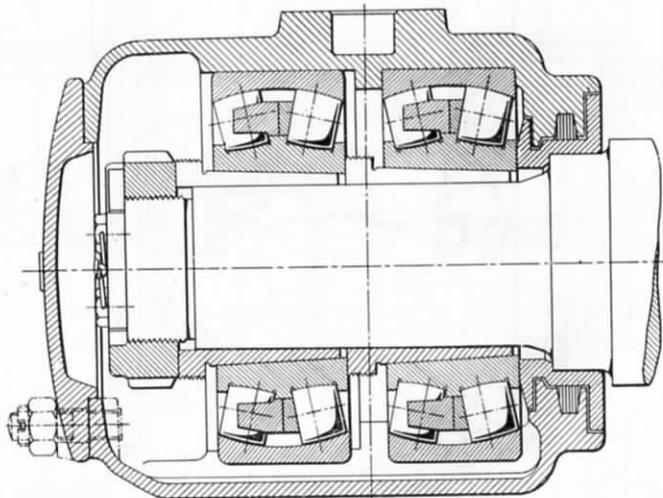
FIG. 72.—S.K.F. ROLLER-BEARING AXLEBOX FOR OUTSIDE JOURNALS.
