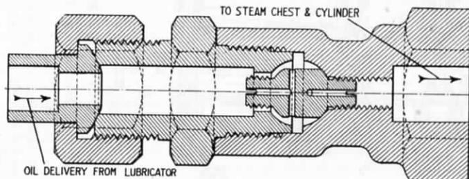
FIG. 223.—STEAMCHEST AND CYLINDER CONNECTION.
