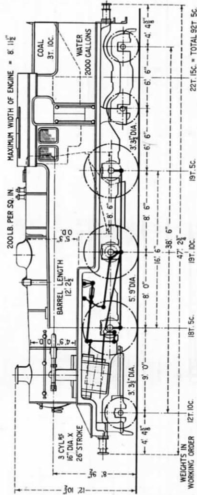
FIG. 290.—"4P" CLASS THREE-CYLINDER 2-6-4 TANK ENGINE, L.M.S.R., WITH TAPER BOILER.
