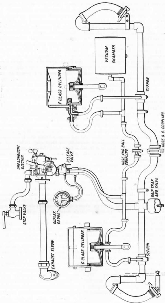
FIG. 183.—GENERAL ARRANGEMENT OF AUTOMATIC VACUUM BRAKE APPLIED TO ENGINE AND TENDER.
