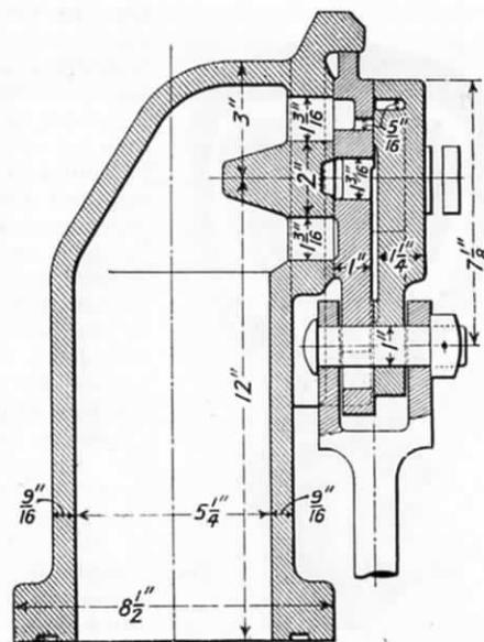
FIG. 37.—DOUBLE-PORTED, FLAT TYPE REGULATOR VALVE.
