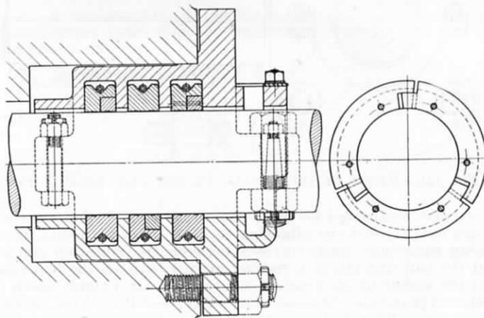
FIG. 123.—ANOTHER TYPE WITH CAST-IRON RINGS.
