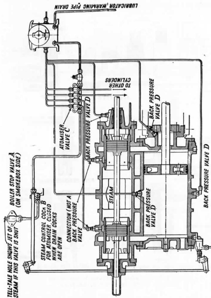
FIG. 236.—SECTION THROUGH LOCOMOTIVE CYLINDER AND STEAMCHEST, SHOWING ARRANGEMENT OF ATOMISER LUBRICATION SYSTEM, L.M.S.R.
