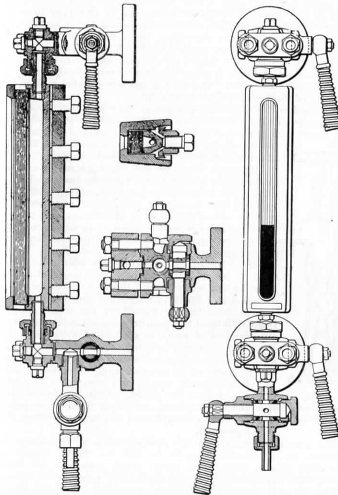
FIG. 48.—DETAILS OF KLINGER REFLEX WATER-GAUGE FITTINGS.
