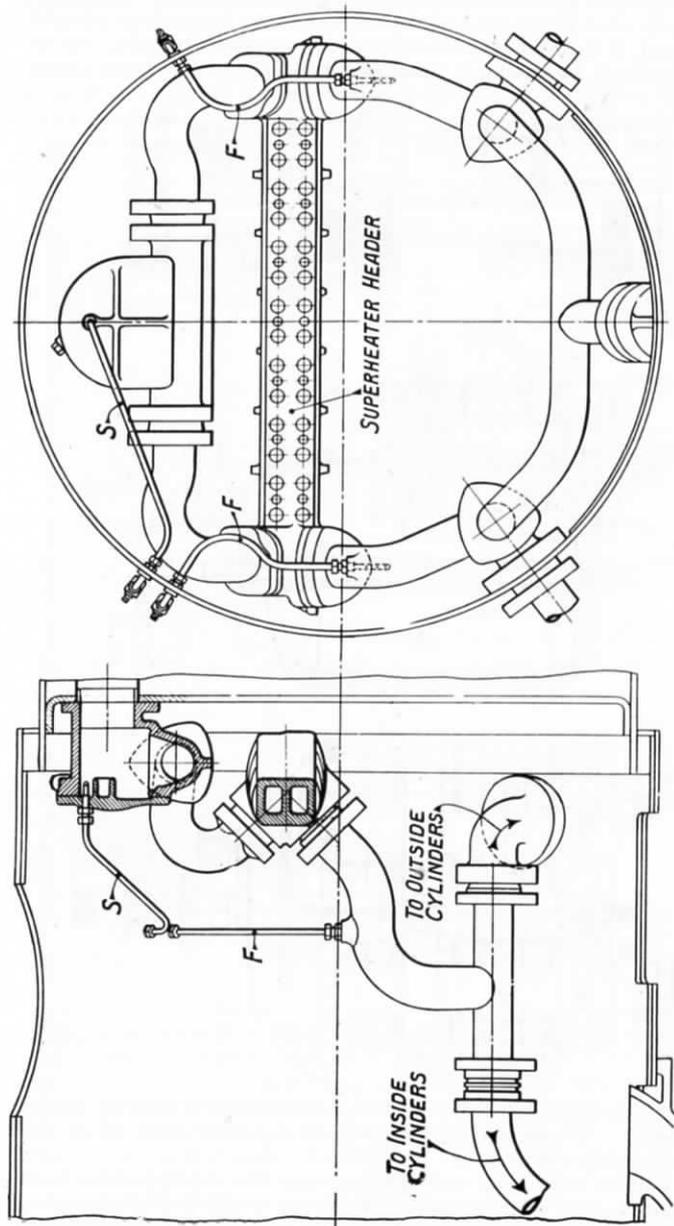
FIG. 235.—LUBRICATION OF FOUR-CYLINDER ENGINES WITH SUPERHEATER, G.W.R.
