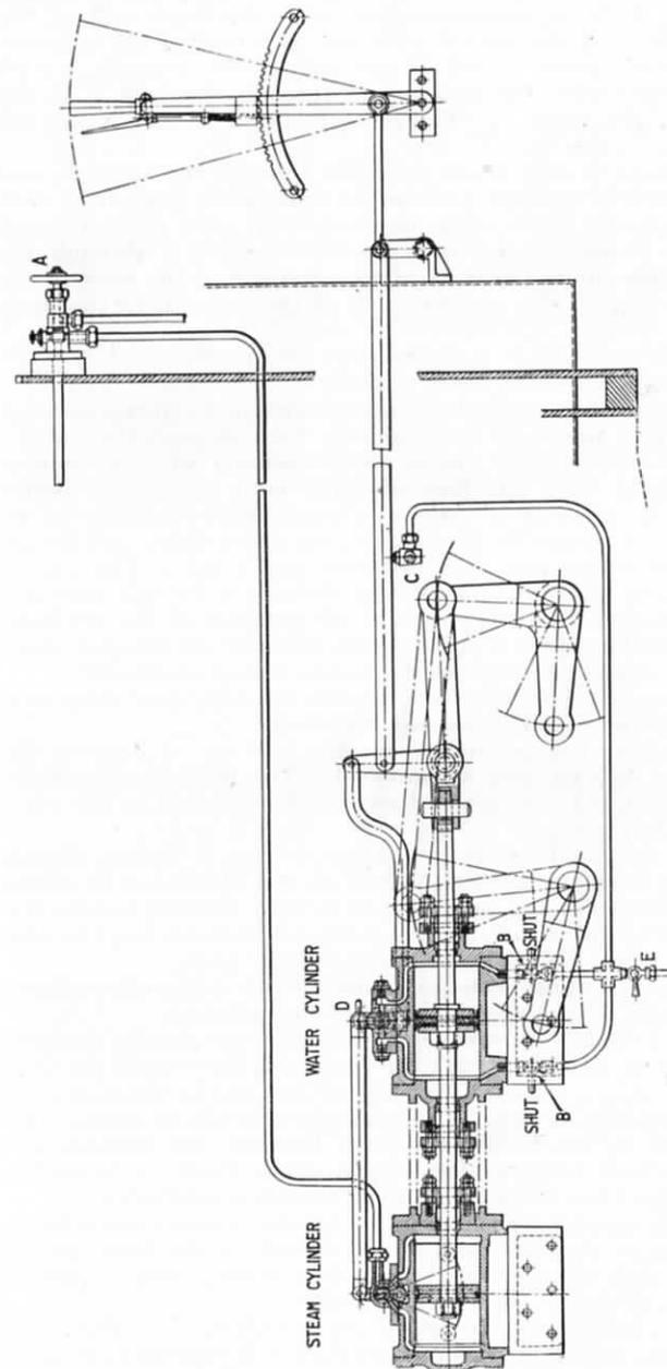
FIG. 96.—DETAILS OF STEAM-OPERATED REVERSING GEAR FOR 0-8-4 TYPE SHUNTING ENGINES, L.N.E.R. (GREAT CENTRAL SECTION).
