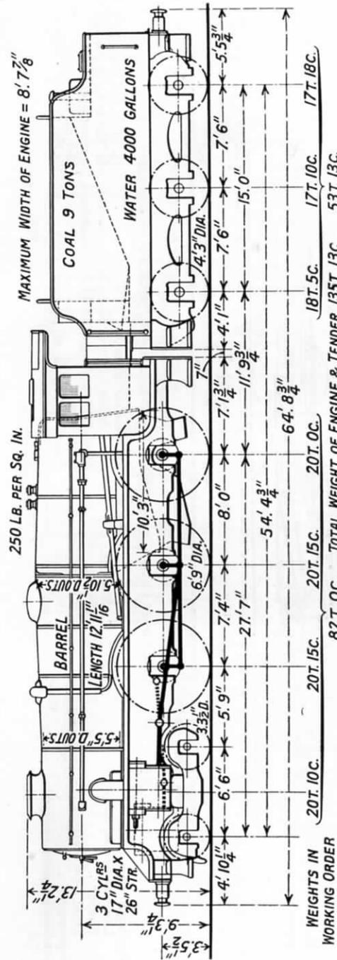
FIG. 289.—"5XP" CLASS 4-6-0 LOCOMOTIVE, L.M.S.R., WITH ENLARGED BOILER AND DOUBLE CHIMNEY.
