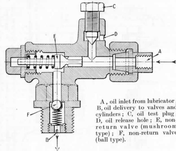
FIG. 227.—COMBINED CHECK AND TEST VALVE FOR WAKEFIELD MECHANICAL LUBRICATORS.
