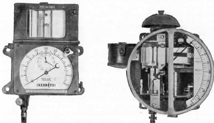
FIG. 242.—THE TELOC AND HASLER SPEED INDICATORS AND RECORDERS FOR LOCOMOTIVES (Hasler Telegraph Works)
