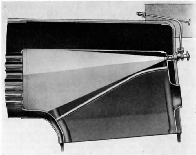
FIG. 23.—SECTIONAL VIEW OF A FIREBOX FITTED WITH CLYDE SOOT BLOWER ON THE BACK PLATE.
