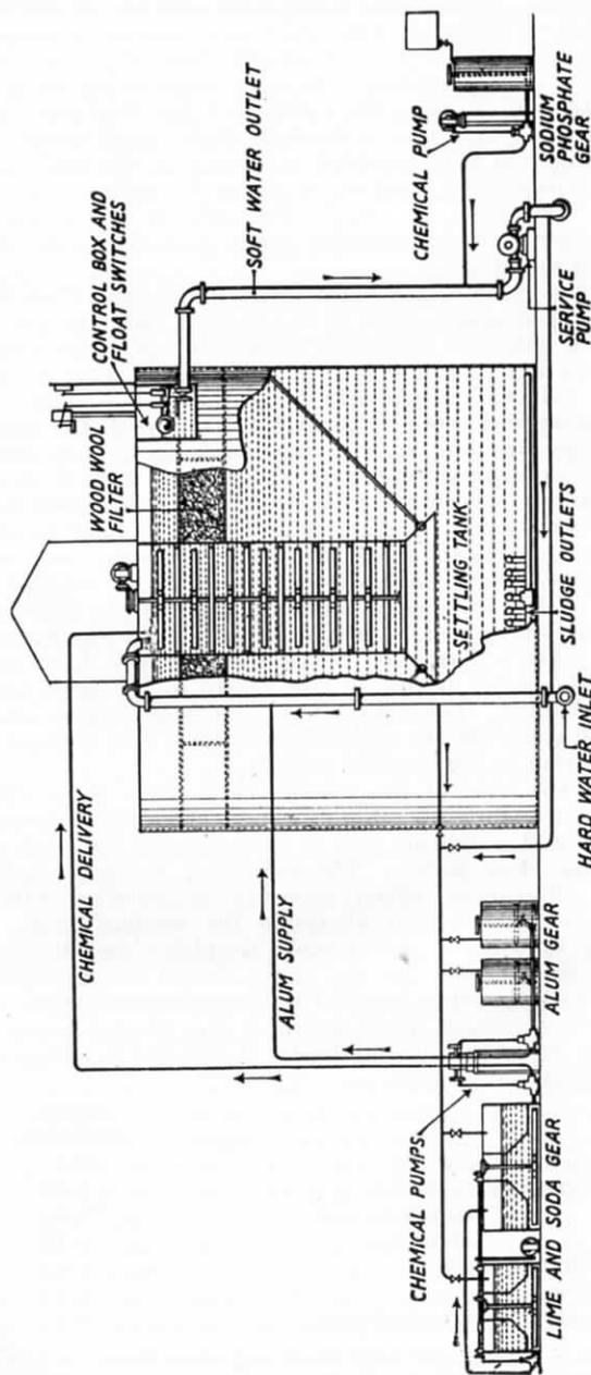
FIG. 29.—KENNICOTT WATER-SOFTENING PLANT AT ECCLES, L.M.S.R.
