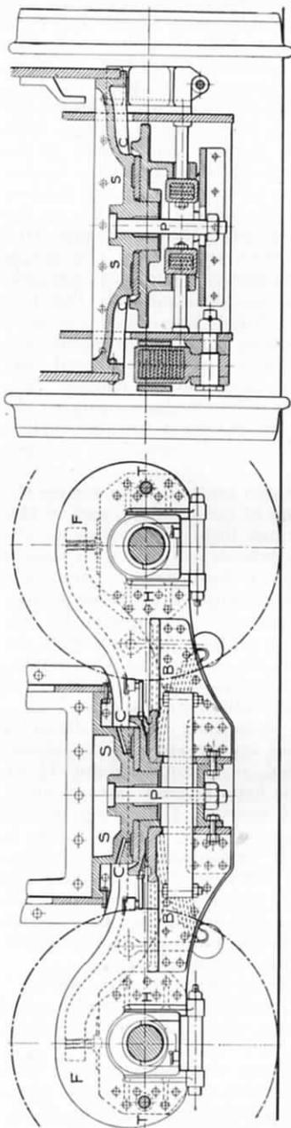
Fig. 83.—DETAILS OF LOCOMOTIVE BOGIE TRUCK.
